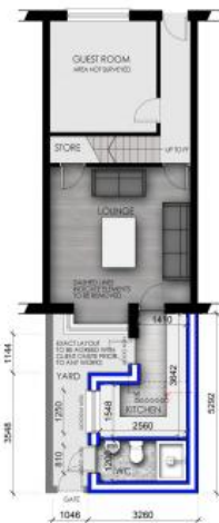
PROPOSED GF PLAN [OPTION A] - 1:100 of A3
