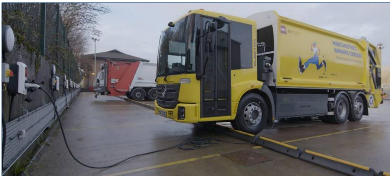
Figure 9-3: One of the City of Manchester's Electra/Mercedes 26 t 300 kWh electric RCVs
