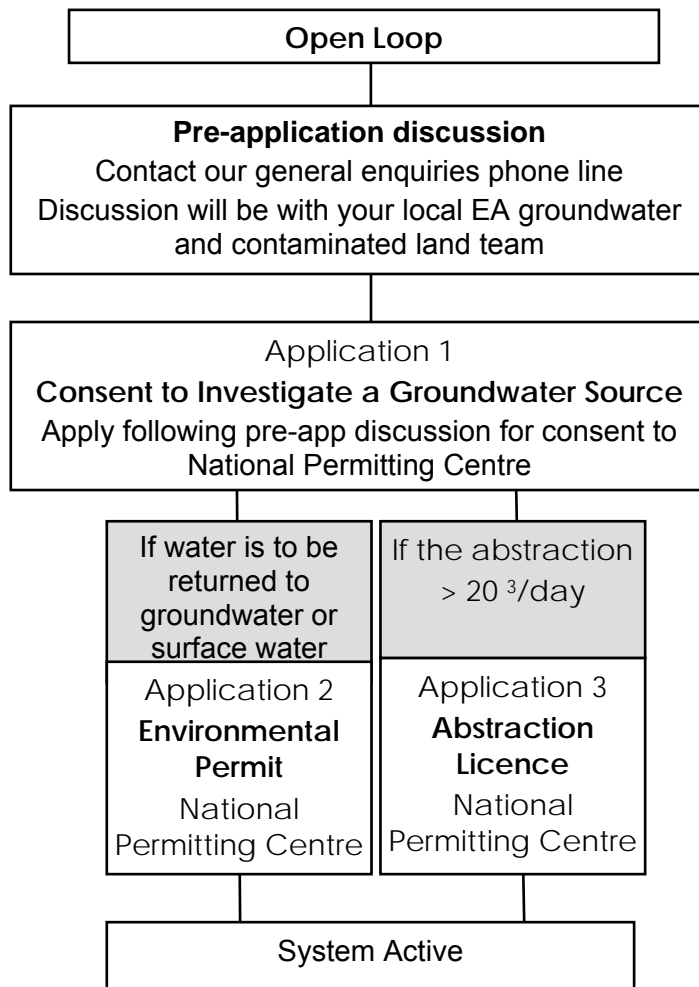
Figure 4.1 Current regulatory pathway for open loop GSHC systems (modified after Fry 2009), showing the separate permitting systems required for different stages.
