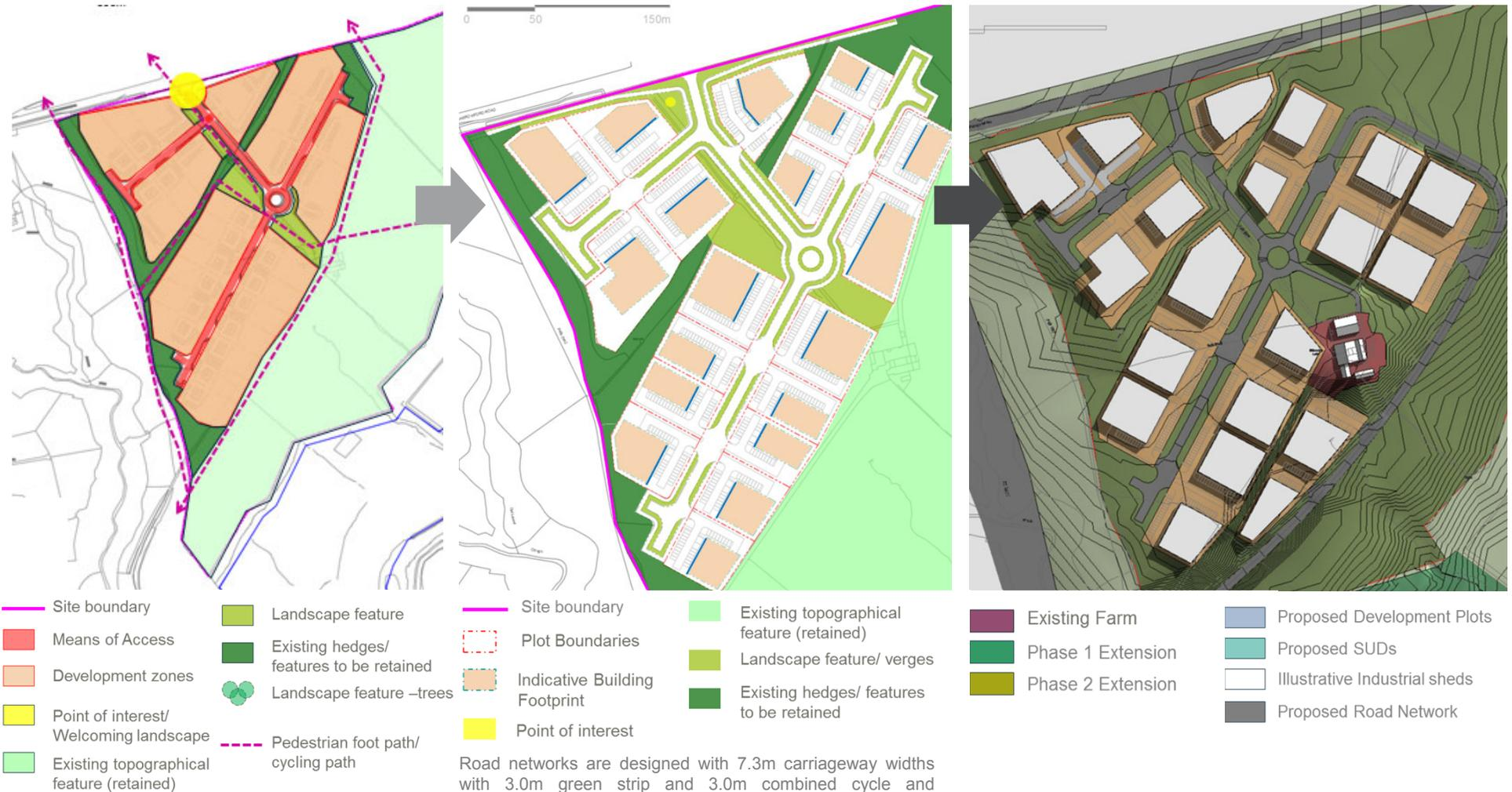
Road networks are designed with 7.3m carriageway widths with 3.0m green strip and 3.0m combined cycle and pedestrian path. Along main spine, landscape feature areas are provided if not a secondary 3.0m green strip.
