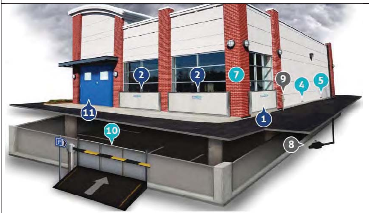
Figure 7.1: Typical Flood Resistance/Resilience Measures for Commercial Development
