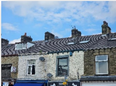
Common issues detracting from the character and appearance of the conservation area, which include modern front facing dormer windows and rooflights, meter boxes, satellite dishes, alarm boxes, security cameras and wiring.
