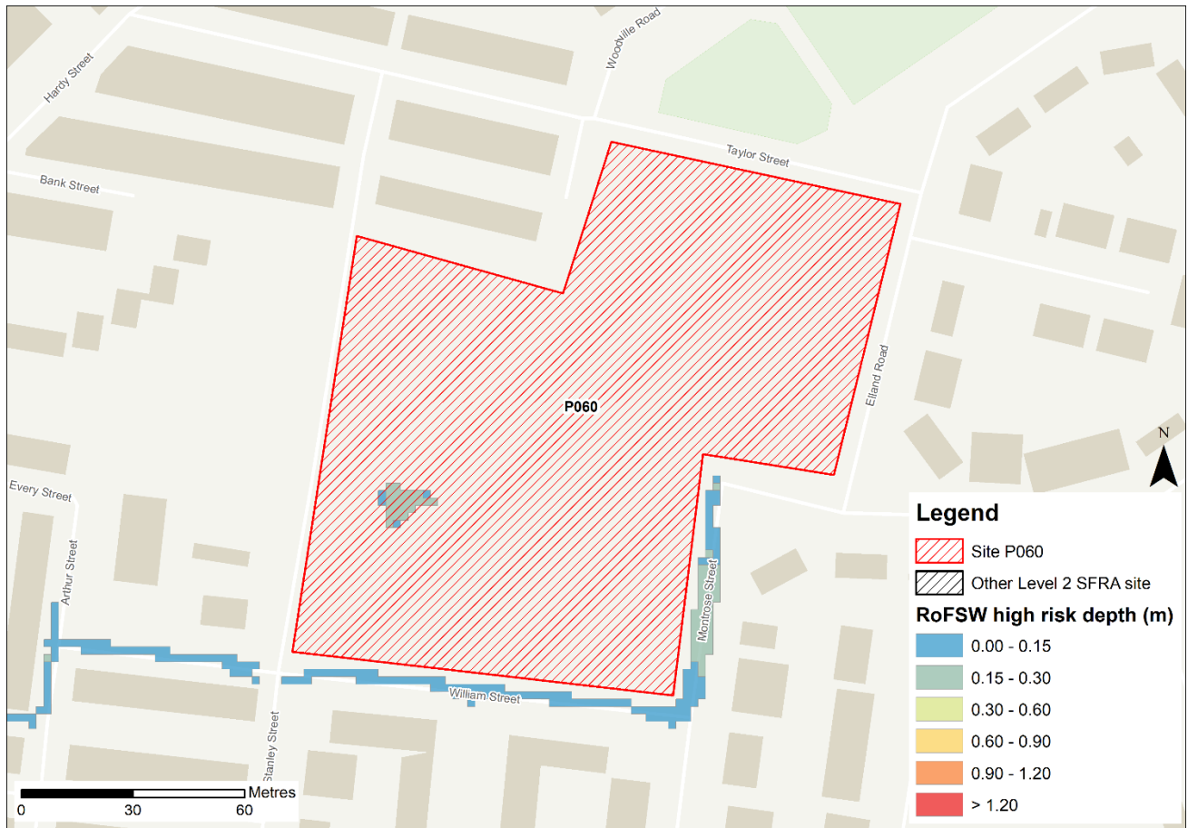
Figure 3-1: high risk event surface water flood depths (Risk of Flooding from Surface Water map)
