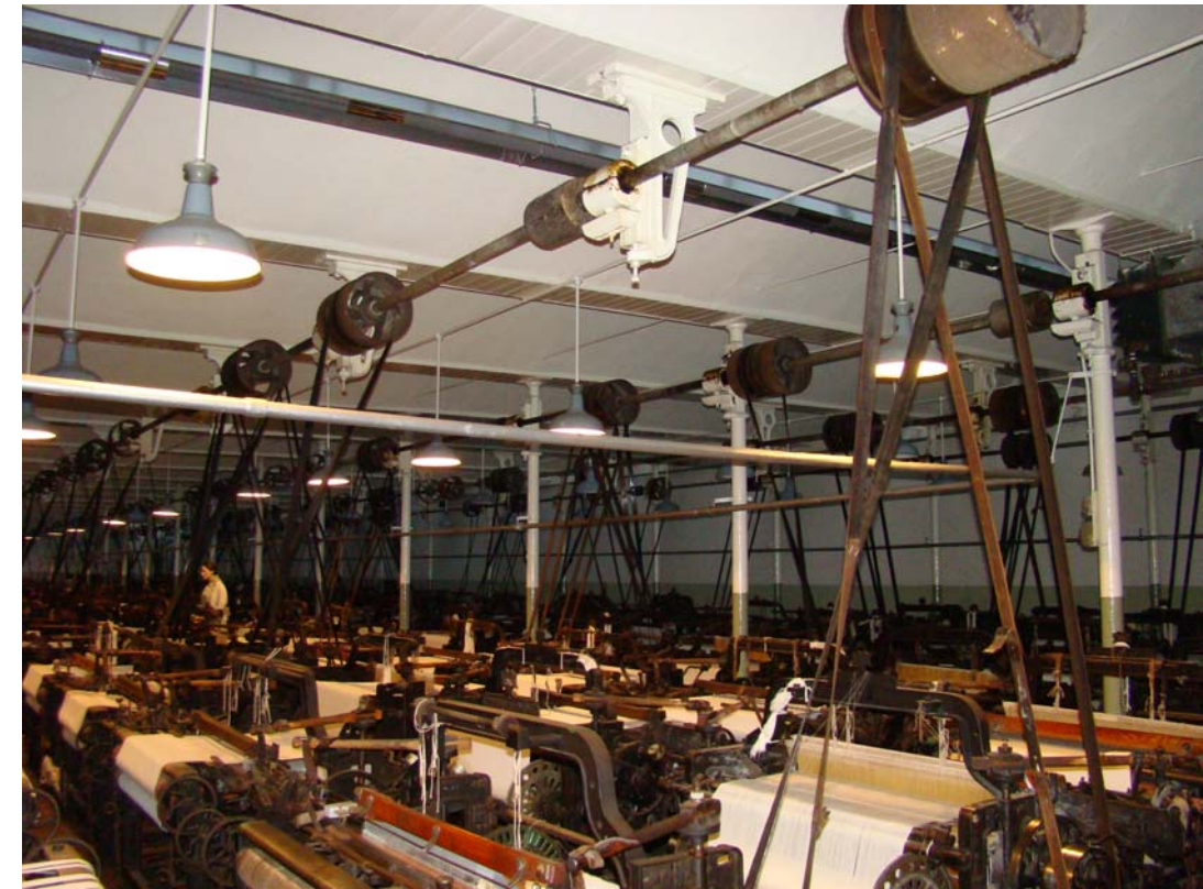
Fig. 27 – Original mechanical services to power looms
