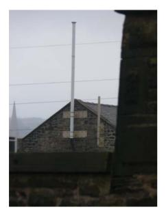
Telecommunication pole with antennae attached to the apex of an existing mill building. The mast is of a slimline design to reduce the impact on the surrounding area. The site could accommodate another similar type pole.
